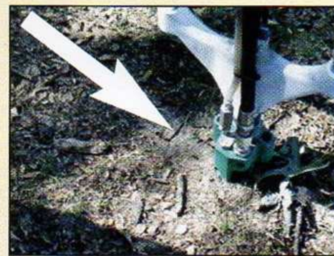
Figure 17. Reducing soil compaction using high-pressure air injector. Cracking of soil indicates some relief from compaction.
